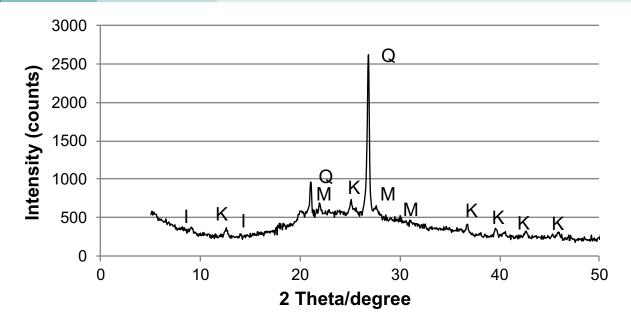
XRD pattern of metakaolin containing waste by-product (MKW). M – microcline, I – illite, K – kaolin, Q – quartz.
