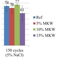
Mixture composition with 10% MKW remained satisfactory concrete properties and could be evaluated as durable after 500 freeze-thaw cycles
