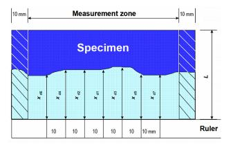
The experimental setup of the test to determine the depth of chloride migration coefficient and the illustration of measurement for chloride penetration depths.
