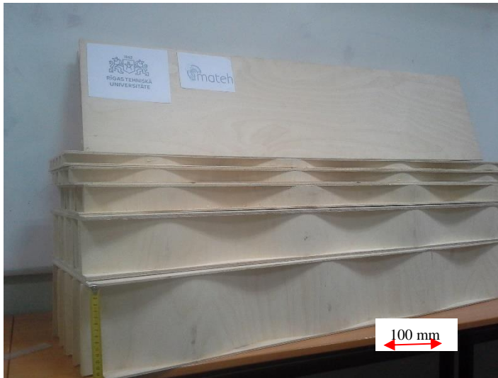
Figure 2. Specimens of plates with cell type hollow core for determination of plates with cell type hollow core. Thicknesses 25 mm; 30 mm; 50 mm; 100 mm and 150 mm.
