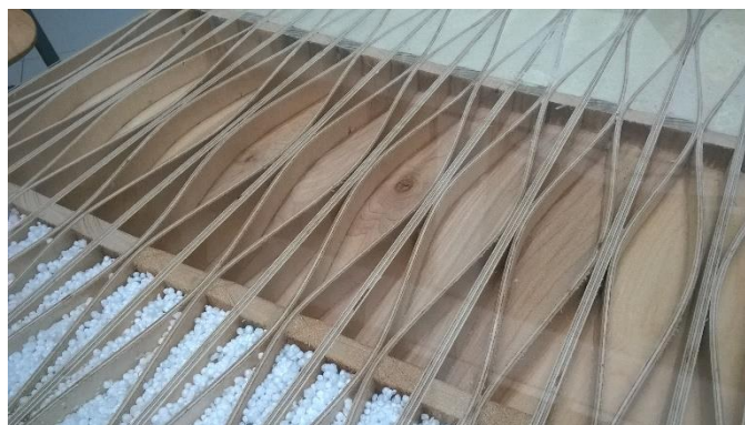
Figure 3. Demonstration model with recycled granulated insulation, without insulation and with polyurethane foam insulation.
