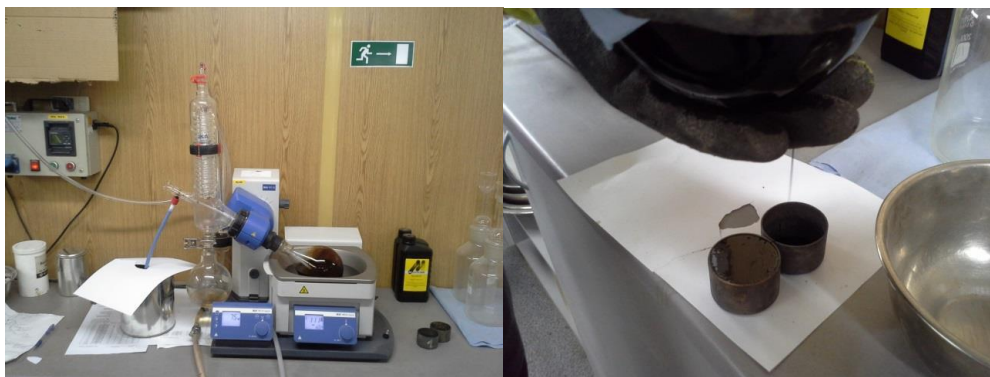
Figure 2.1. Bitumen recovery with rotary evaporator.
