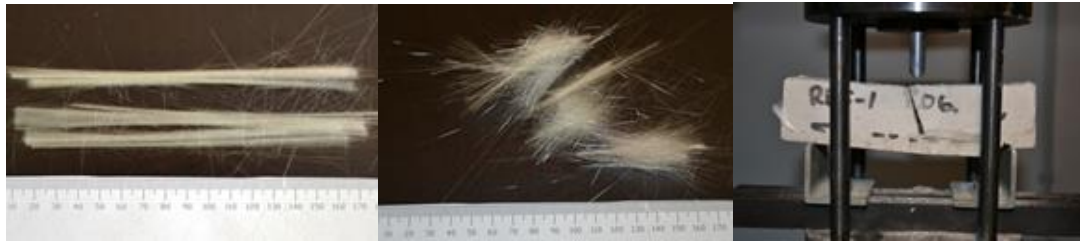
Figure 1.1 Fiberglass bundles made of fiberglass siftings; disperse reinforcements and specimens made with bundle reinforcement in the stretched zone after the bending strength testing.
