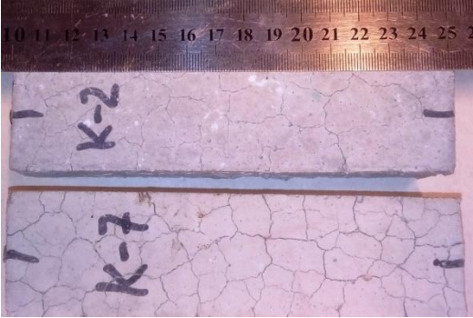
Figure 1.6 Network of microcracks related to alkali-silica reaction on samples with K-type micro-fillers.
