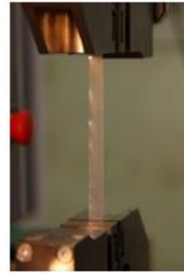
Fig. 12. Tensile testing of the film
