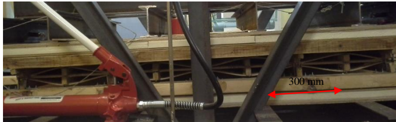
Figure 4. Part of the equipment for production of cell type hollow core in compressed state
