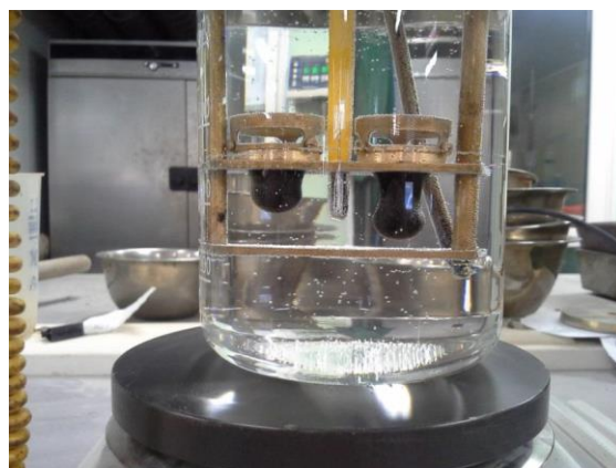
Figure 2.2 Bitumen softening temperature testing.
