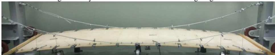
Figure 6. Physical model with deck resisting longitudinal loads
