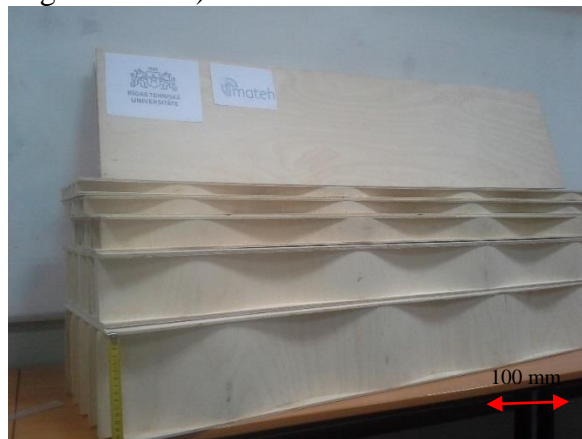
Figure 1. Specimens of plates with cell type hollow core for determination of plates with cell type hollow core. Thicknesses 25 mm; 30 mm; 50 mm; 100 mm and 150 mm.
