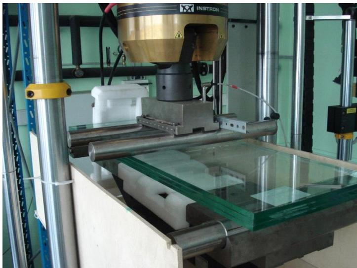
Fig.1. A laminate glass sample tested in bending (INSTRON 8802)
