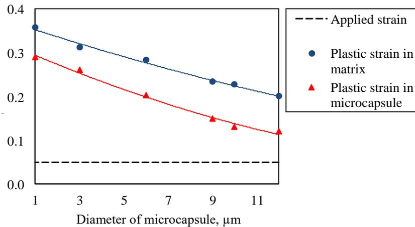
**Figure 9.** Dependences of strain upon diameter of capsule.
