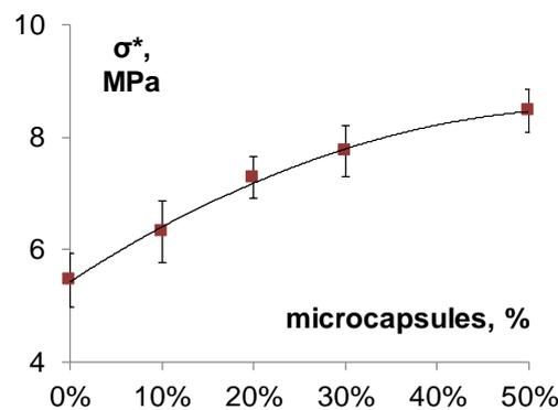
**Figure 3.** Yield strength of PVA matrix composite specimens for different amount of microcapsules by weight.
