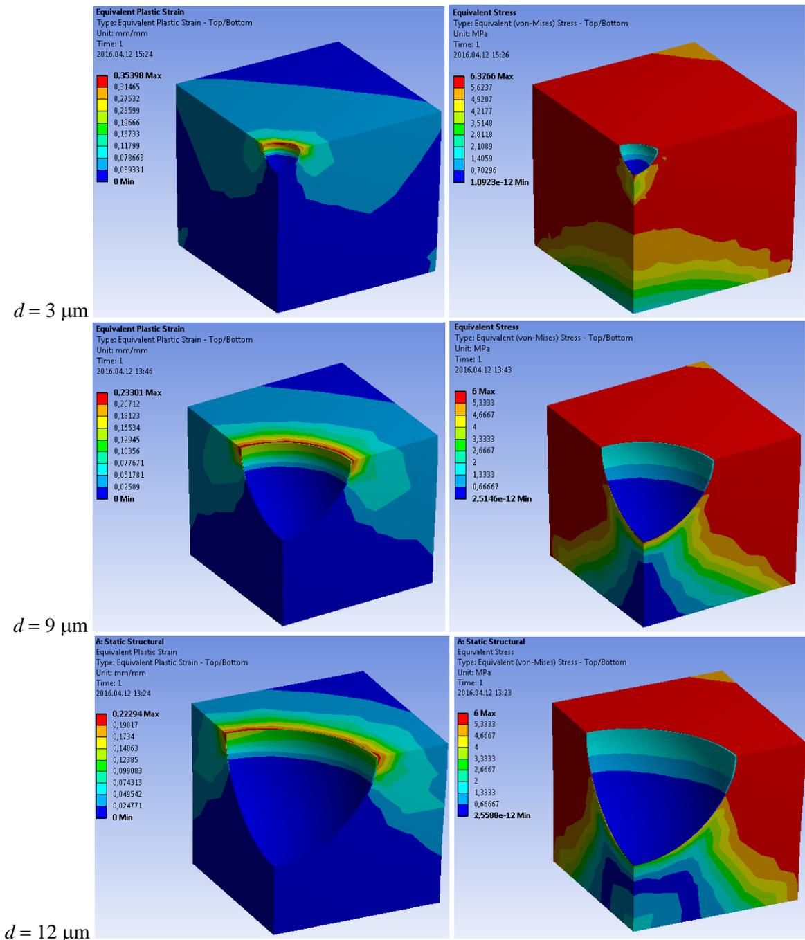
**Figure 8.** Equivalent plastic strain and equivalent stress of RVE as the applied strain 0.05.
