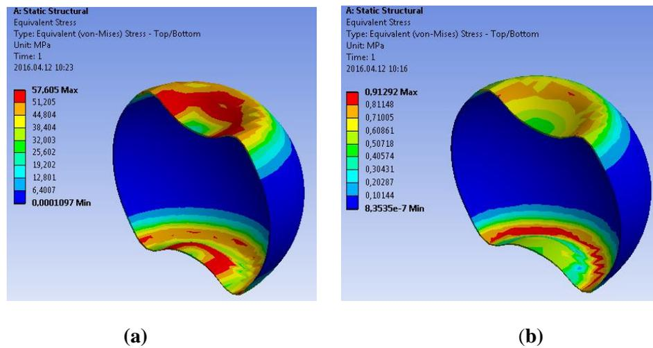
**Figure 6.** Von Mises stress in nitrocellulose (a) and MF resin (b) balls under displacement 7.5 mm.
