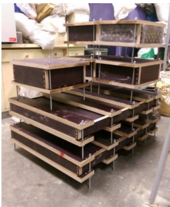
Fig. 2: Moulded samples for mechanical and reaction to fire tests
