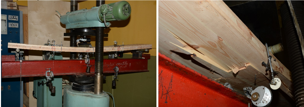
Fig. 6. (a) Plate under loading nearly collapse stage; (b) Collapse of CLT slab.
