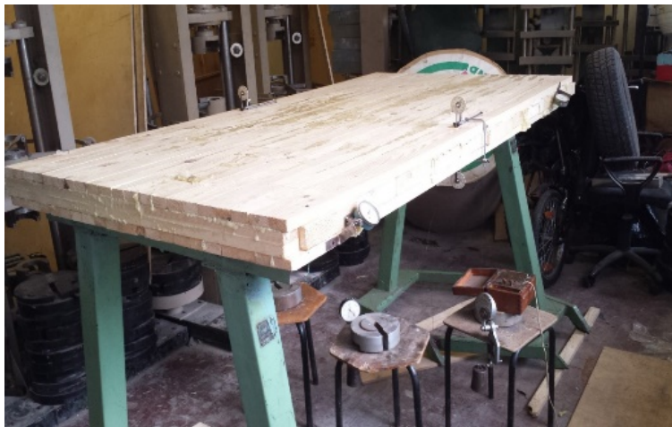
a) – CLT plate before loading
