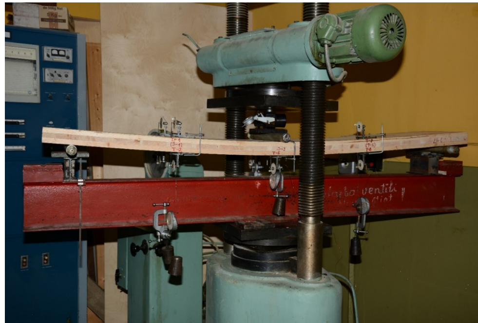
Plate under loading nearly collapse stage
