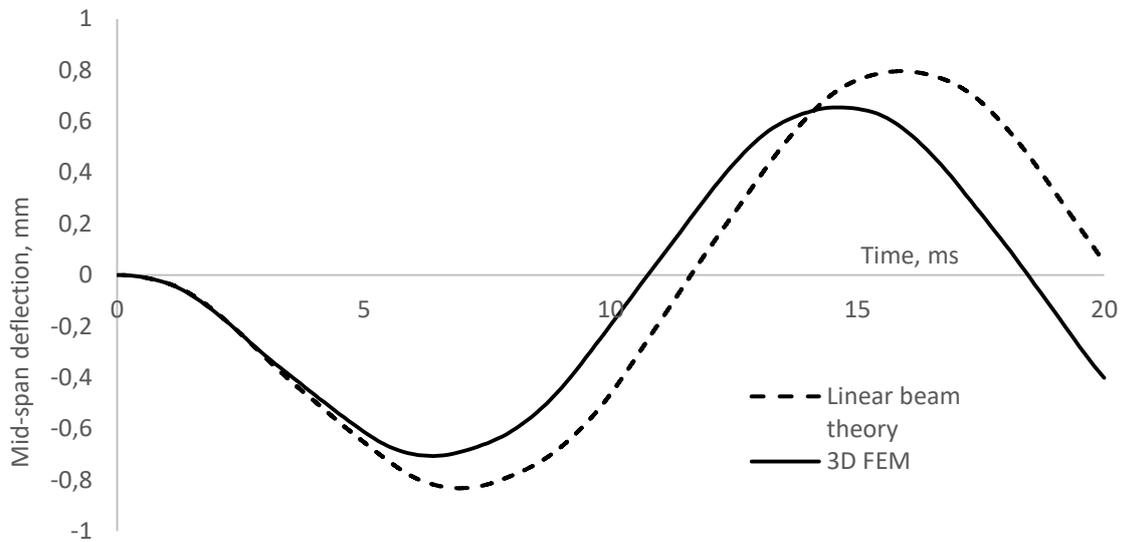
**Figure 3.** Deflection change in time, 3-layers, all in one direction. Applied load  $p_{max}=1$  KPA,  $t_0=10$  ms.
