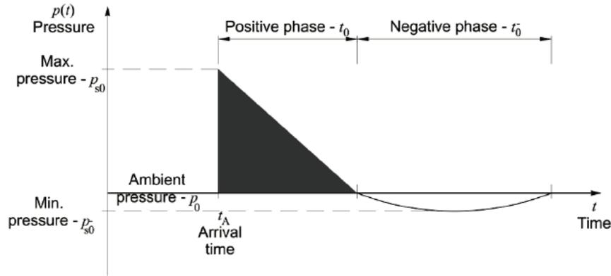
Figure 2. Pressure-time profile of the explosion wave [14].
