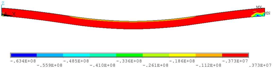
**Figure 9.** Axial stress distribution after failure at  $t=169$  ms.
