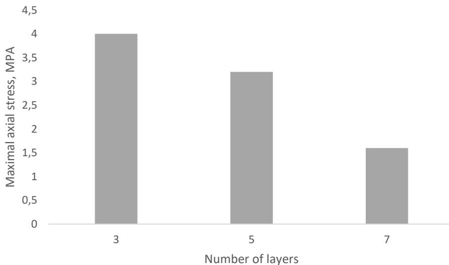
**Figure 6.** Stress in middle of span in layer of weave contact, depending on layer count. Applied load  $p_{max}=1$  KPA,  $t_0=10$  ms.
