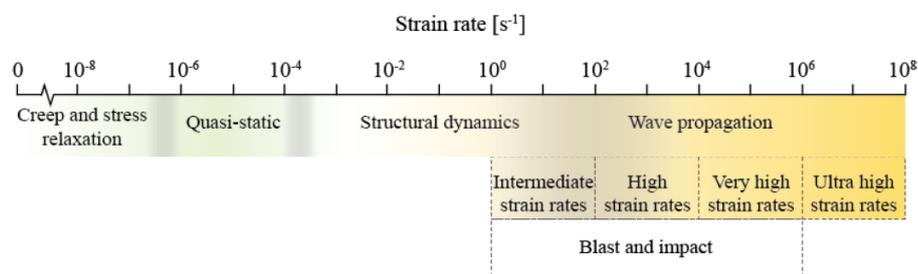
**Figure 1.** Structural problem classification depending on strain rate. Figure taken from [4].
