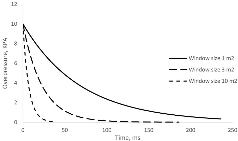
**Figure 11.** Pressure-time curves depending on size of openings.
