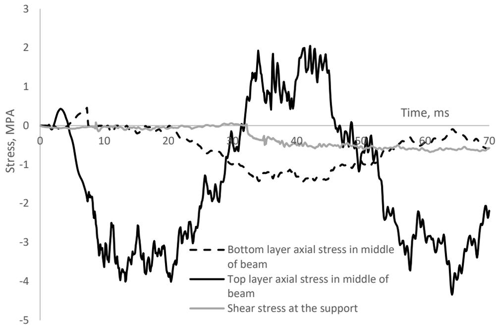
**Figure 5.** Axial stress change in time. Applied load  $p_{max}=1KPA$ ,  $t_0=10$  ms.
