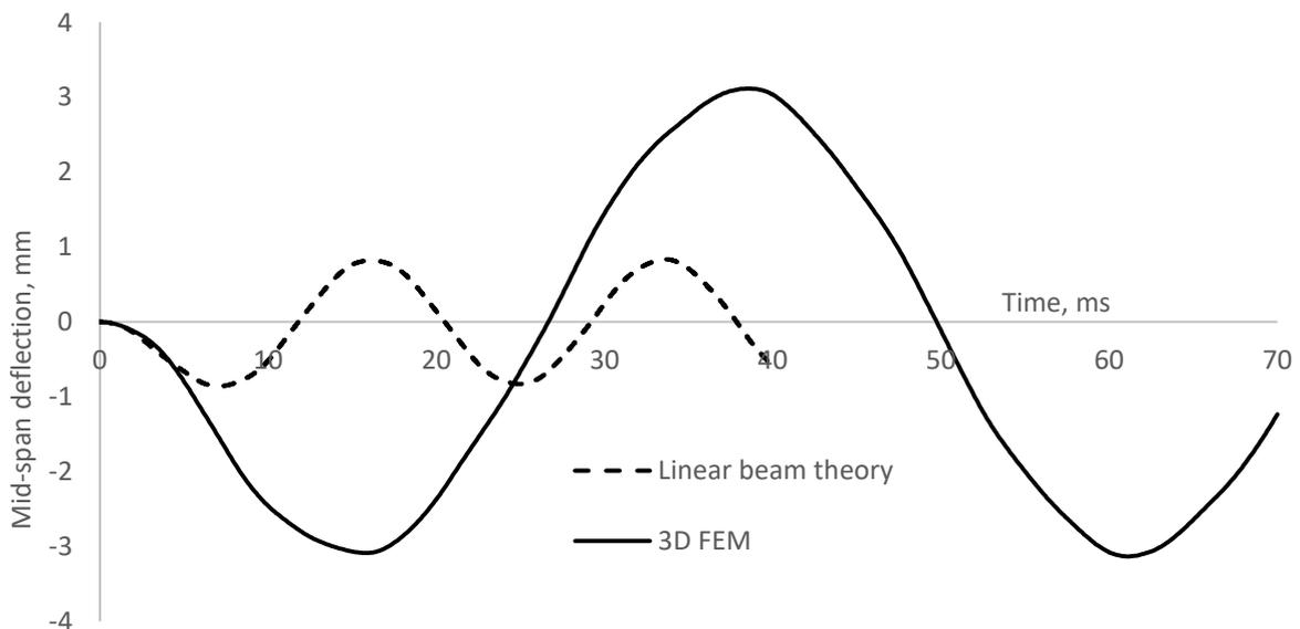
**Figure 4.** Deflection change in time, 3-layers, middle layer in perpendicular direction. Applied load  $p_{max}=1$  KPA,  $t_0=10$  ms.
