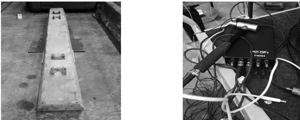
Figure 2. Modal analysis test setup. Left: concrete sleeper on a rubber mat, right: testing equipment.
