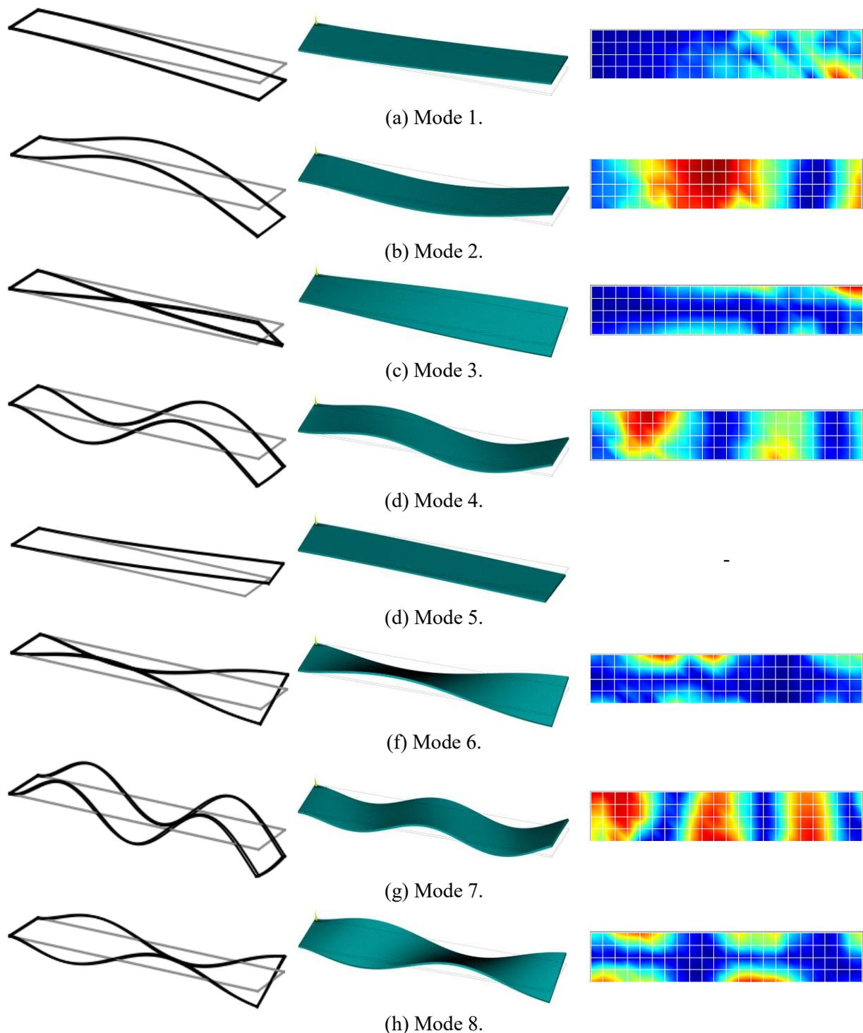
Figure 3. Modes shapes from PD simulation (left), FE simulation (center), laser vibrometer (right).
