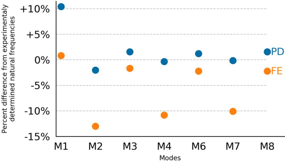
Figure 2. Percent difference between natural frequencies determined experimentally and simulated in peridynamics and finite-elements.
