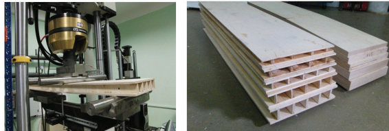
Fig. 3: Test set-up for bending test. Prototyped sandwich panels in comparison with conventional plywood boards.
