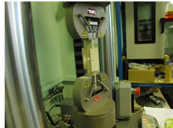
Specimen placed in the testing machine (Instron 3000).
