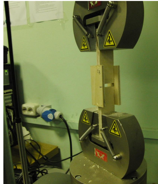
Specimen placed in the testing machine (Instron 3000).
