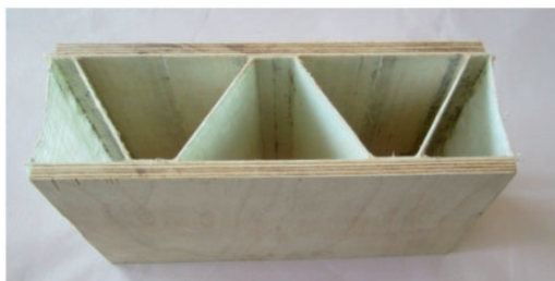
Figure 5. Sandwich panel with plywood face sheets and GF/PP core (PW_GF).
