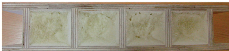
Figure 3. Plywood sandwich panel vertical stiffener and foam core (PW_F).
